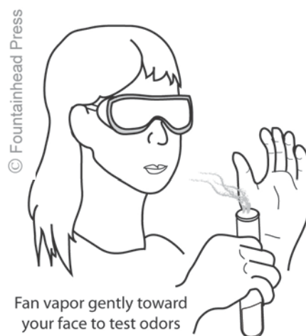
Figure 1. Proper technique for detecting vapors/odors from test tube.
